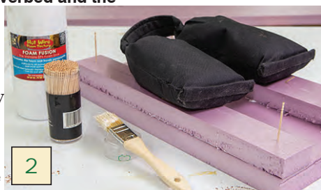
The foam pieces are glued together using Hot Wire Foam Factory Foam Fusion foam glue and held in place with toothpicks and weighted down overnight to allow the glue to fully cure.
