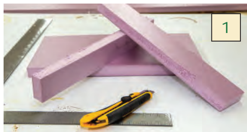
Three pieces of one inch EPS foam are cut to size to form the riverbed and the two banks.
