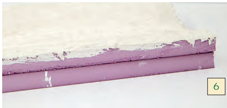
To smooth out some of the roughness caused by the fibrous compound, I applied a thin layer of USG Hydrostone using a disposable paint brush. This was allowed to fully dry.
