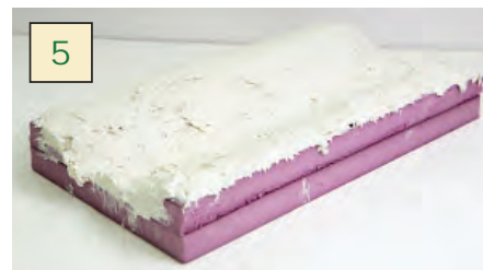
The mix is applied with a putty knife roughly matching the contours of the two banks. The applied goop is allowed to fully dry for several days. The thinner the layer, the better. You do not want to mask the contours.
