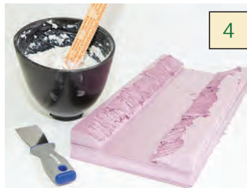
A mix of SCULPTAMLD modeling compound and 1/4 cup of USG Hydrostone is mixed with water to a goop-like consistency.
